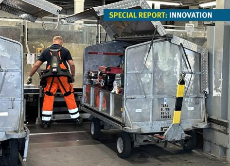
The AI-based power suits were developed specifically for repetitive lifting tasks that place heavy strain on the lower back.
